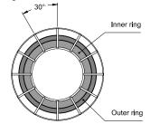
The sensor head can tilt about one of its axes if it is desired to displace the detection area.
